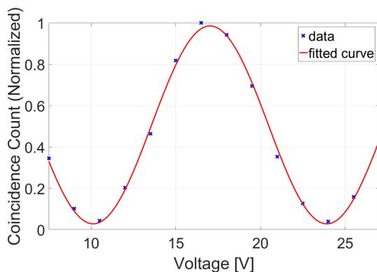
Figure 1: Normalized coincidence count as a function of the voltage applied on a piezo to control the phase.
